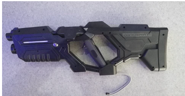
Figure 3a.4: A Rifle Gun Attachment for HTC Vive Motion Controller. The attachment helps the HTC Vive Motion Controller to feel and handle more like a rifle fig:hyperphysicality-hardware-accessories2
