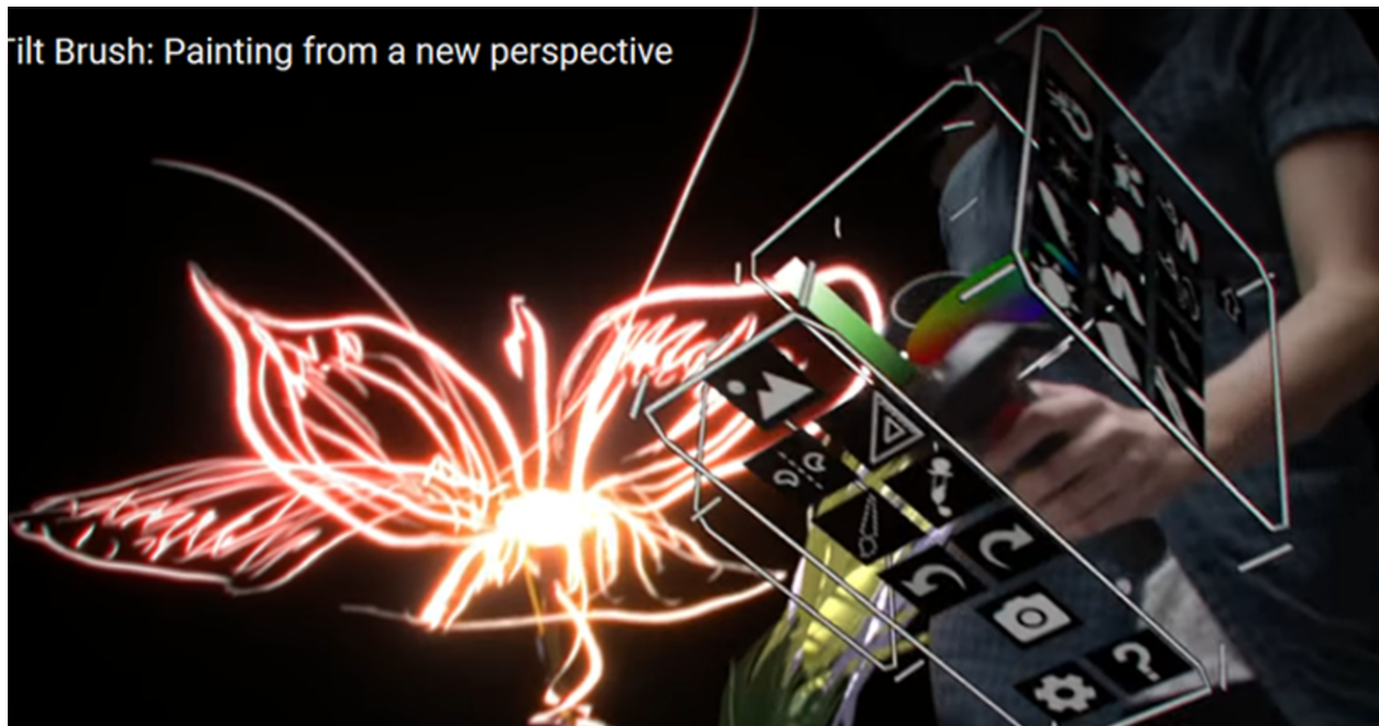
Figure 3a.7: Mixed reality image of Google’s VR Drawing Application Tilt Brush. It depicts virtual interfaces attached to the physical VR controller
